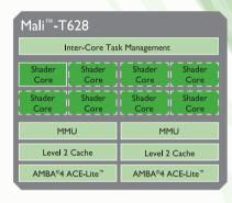
The ARM Mali-T628 GPU offers scalability from one to eight cores – providing up to twice the graphics and GPU Compute performance compared to the Mali-T624 GPU. The Mali-T628 shares key API support with the other products in the Mali-T600 Series – including OpenGL\* ES 1.1, 2.0 and 3.0, DirectX\*\* 9, DirectX 11, OpenCL 1.1 Full Profile and Google Renderscript.
